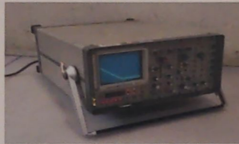
Figure 2. The USIP-12 Ultrasonic Flaw Detector supplied by KCP used in the first testing trials. These trials were inaccurate.
